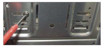
**6**. Push in the reservoir flush with the front of the PC case and use the 4 provided screws to fix it securely in place.
