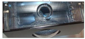
**4.** Start to fill the reservoir, it may help to use a funnel to avoid spillage. Keep filling the reservoir until the liquid stops draining into the tubing.
