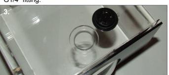
3. When you are happy that all the components in the loop are securely connected, remove the filler cap by using a small coin and turning anticlockwise.
