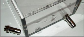
**1**. Screw the G1/4" fittings to the inlet and outlet making sure the o-rings are compressed. 1/2" barbs are used in the photo but you can use any type of G1/4" fitting.
