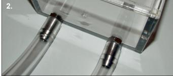
**2.** The reservoir should be connected to the pump, water-blocks and radiator in a loop. When you connect the tubing it is important that the reservoir outlet is connected to the pumps inlet.
