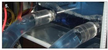
**5**. Turn on the pump and as the reservoir drains top up the water level. Leave the pump running to remove all the air from the system. When all the air has been removed replace the filler cap and turn it clockwise to seal the reservoir.
