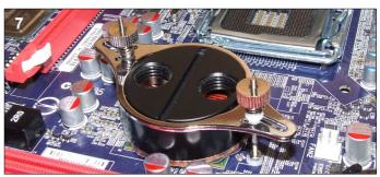
**7.** Place a washer over each rod followed by a spring. Finally screw the two knurled nuts onto the threaded rod until the springs are 50% compressed. The chipset block is now ready for use, it is advisable to check temperatures on the first boot.
