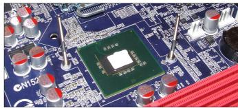
**5.** Make sure the nuts on the top side of the board are tight and the rods are secure. Then apply a thin layer of thermal paste to the chipset core.
