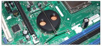
**6**. Step 4 and 5 should be repeated using the second wire clip on the two remaining loops. The chipset block is now ready for use, it is advisable to check the chipset temperature on the first boot.
