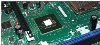
**2.** Clean any residue left over from the heatsinks thermal pad and apply a thin layer of thermal paste to the chipset core.
