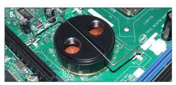
**5**. With one hand on the waterblock take the other end of the wire clip and hook it onto the opposite loop.
