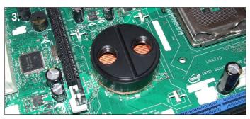
**3**. Remove the protective film from the waterblocks base and place the block on the chipset. The channel on the top should be facing in the direction shown above.
