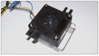
**3**. Use the 4 supplied screws to attach the acrylic top to the pump, tighten the screws until the large o-ring is compressed. It is best to double check that the center of the blue impeller lines up with the center of the tops inlet port.
