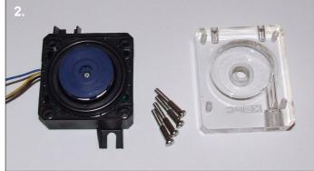
**2.** Place the acrylic top on to the DDC pump making sure the center of the pump lines up with the center of the acrylic top.
