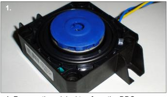
**1**. Remove the original top from the DDC pump by unscrewing the four screws on the base of the pump. Place the o-ring back onto the pump.
