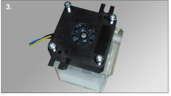
**3**. Use the 4 supplied screws to attach the reservoir to the pump. Tighten the screws until the pumps o-ring is compressed.
