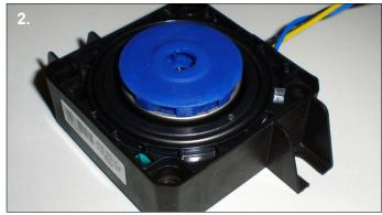
**2.** Remove the original top from two the DDC pumps by unscrewing the four screws on the base of the pump. Place the o-ring back onto each of the pumps.
