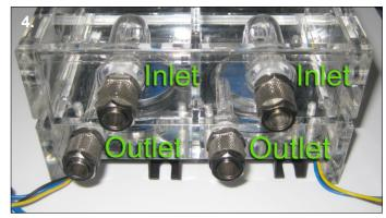
**4.** Now screw the G1/4" fittings to the inlets and outlets making sure the o-rings are compressed. Push the LED or LED's into any of the three 5mm holes on the back of the reservoir. The pump is now ready to be connected to your other watercooling components and leak tested before being fitted into two 5.25" drive bays.
