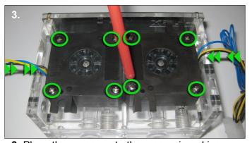
**3**. Place the pumps onto the reservoir making sure that the o-rings stay in place. The pumps should be orientated so the wires are on the outer sides of the reservoir. Use the 8 long M4 screws to attach each pump to the reservoir, tightening them until the large o-ring is compressed.
