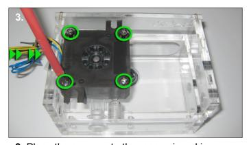
**3**. Place the pump onto the reservoir making sure that the o-ring stays in place. The pump should be orientated so the wires are on the outer side of the reservoir. Use the 4 long M4 screws to attach the pump to the reservoir, tightening them until the large o-ring is compressed.
