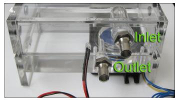
**4.** Now screw the G1/4" fittings to the inlet and outlet making sure the o-rings are compressed. Push the LED or LED's into any of the three 5mm holes on the back of the reservoir. The pump is now ready to be connected to your other watercooling components and leak tested before being fitted into two 5.25" drive bays.
