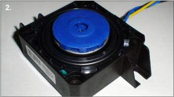
**2.** Remove the original top from the DDC pump by unscrewing the four screws on the base of the pump. Place the o-ring back onto the pump.
