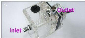
**4.** Use an adjustable spanner to connect the G1/4" fittings of your choice to the inlet and outlet. The reservoir is now ready to be connected to your other components and leak tested.
