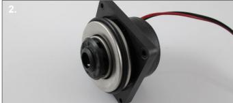
**2.** Push the plastic mounting plate over the back of the pump. The circular cut-out on the plastic should be facing the front. Now place the new o-ring in the circular cut-out around the pump.
