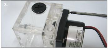
**3**. Line up the pump and plastic mounting plate with the 4 screw holes on the back of the reservoir and attach it using four M4 screws. Make sure the o-ring is compressed.
