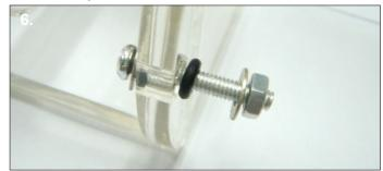
**6**. If you attach the reservoir to your case using the screws please attach them in the following order. Screw > washer > o-ring > reservoir > o-ring > case > washer > nut.
