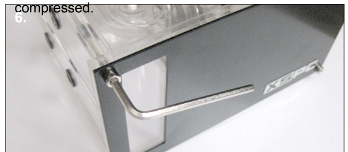
6. Choose a faceplate for the front of the reservoir and use the 4 allen head screws and the allen key tool to attach it.
