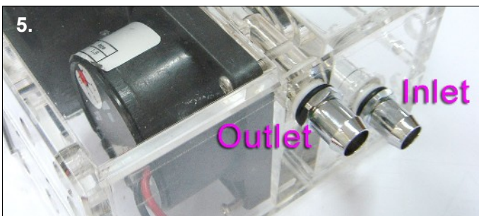
5. Use an adjustable spanner to connect the G1/4" fittings of your choice to the inlet and outlet. The reservoir is now ready to be connected to your other components and leak tested.
