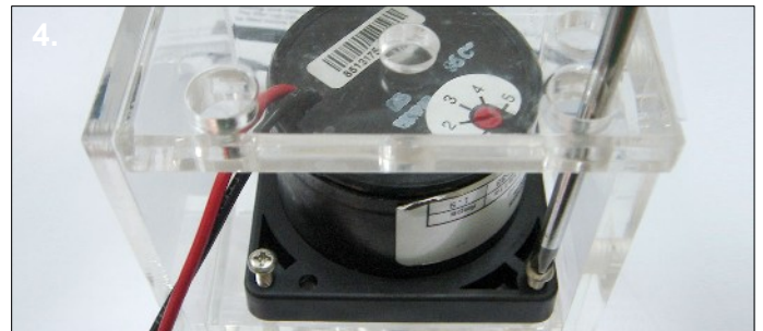
4. Lift the pump through the bottom of the reservoir and line up the 4 screw holes. Now take a screw driver and tighten each screw through the holes on the reservoirs side. Check the o-ring is compressed.
