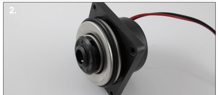
2. Push the plastic mounting plate over the back of the pump. The circular cut-out on the plastic should be facing the front. Now place the new o-ring in the cut-out and around the pump.
