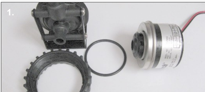
1. Disassemble the D5 pump by unscrewing the circular bracket anticlockwise. Put the bracket, o-ring and pump front to one side, they're not needed.
