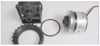
3. Disassemble the D5 pump by unscrewing the circular bracket anticlockwise. Put the o-ring to one side, you will need this in step 5..
