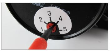
7. The dial on the back of the pump can be used to set the pump speed. 5 being full power and 1 being the lowest noise level. The speed setting on each pump should be matched.
