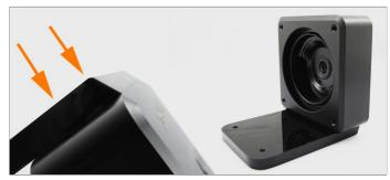
2. Use the two small screws to attach the acrylic stand to the D5 top. Two of the longer screws and the nuts can be used later to secure the stand to your case.
