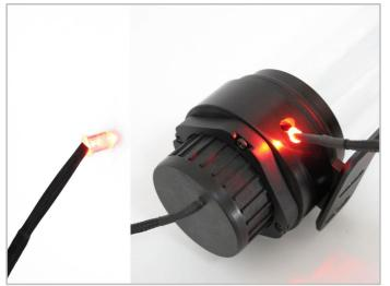
**3**. When fitting the LED, slightly kink the LED wire and push the LED into the hole on the base of the reservoir. You might need to twist the LED slightly until it slots into place.
