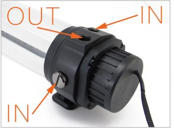
1. The pump has one outlet and two inlets. Attach the G1/4" hose fittings to your ports of choice and use the G1/4" plug to block the unused port..
