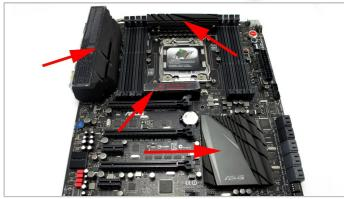
2. Turn the board back over and slowly remove the stock heat sink from the board. You should be careful not to damage any components on the board.
