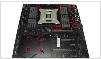
1. Turn the board over and remove the thirteen screws highlighted above. Keep these to one side, they will be needed in step 5.
