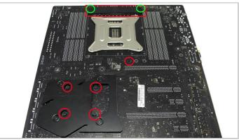
5. With one hand on the blocks, turn the board back over. Refit the five original screws to positions marked in red and the M2x8mm screws and washers to positions marked in green.
