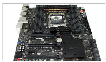
**4**. Remove the plastic film from the A and B water blocks and carefully place them into position on the motherboard. You should check the thermal pads are still in position.
