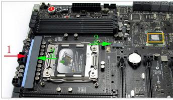
3. Remove the film from both sides of the thermal pads. Place the blue pad on position 1 and the grey pads on positions marked 2. Now apply K2 paste to the chipset.
