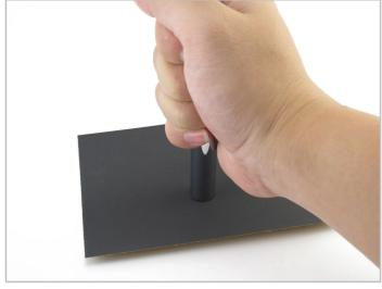
8. Finally, rub the end of the tube back and forth against the sandpaper to remove any rough edges.
