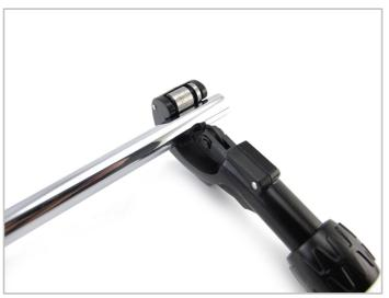
1. Measure the length of the cut your need and mark it on the tube. Now place the metal tubing into the cutting tool, so that the tube sits between the two rollers and the blade.
