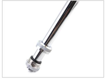
9. Once the sharp edge of the tubing has been removed you can insert the end of the tube into the fitting. The tube must push past the two internal o-rings and finally be sealed by the outer compression o-ring.
