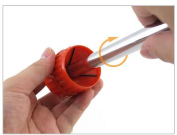
7. Insert the cut end of the tubing into the chamfer tool and rotate it clockwise. This will clean the outside edge of the tubing.
