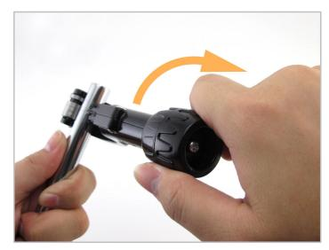
5. Repeat the two previous steps, rotating the tool around the tube and then gradually tightening each time.
