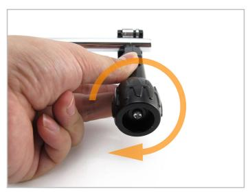
2. Line the cut mark up with the blade and tighten the handle on the cutting tool until the blade is in contact with the tube.
