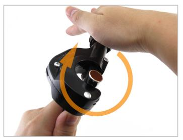
3. Rotate the cutting tool around the tubing several times.
