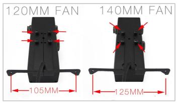
3. The bracket can be used with both 120, or 140mm fan mounts. If you are using 120mm fans use the outer holes and for 140mm fans, use the inner holes.
