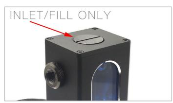
2. The fill cap port can also be used as an inlet with the use of a M20 to G1/4" adapter. The fill cap cannot be used an an outlet.
