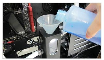
6. When the lon is connected to all other components, you can remove the fill cap and fill the reservoir. The coolant level should be at the top of the window.
