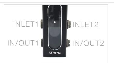
1. The Ion has four G1/4" ports. The bottom two can be used for either an inlet or outlet. Attach the hose fittings to your ports of choice. The unused port can be blocked with the provided G1/4" plugs.
