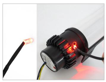
3. When fitting the LED, slightly kink the LED wire and push the LED into the hole on the base of the reservoir. You might need to twist the LED slightly until it slots into place.
