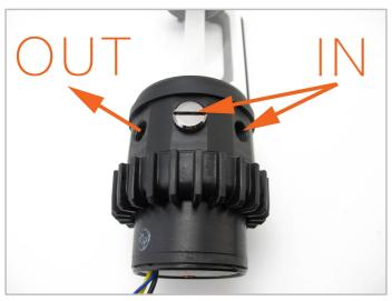
1. The pump has one outlet and two inlets. Attach the G1/4" hose fittings to your ports of choice and use the G1/4" plug to block the unused port..
