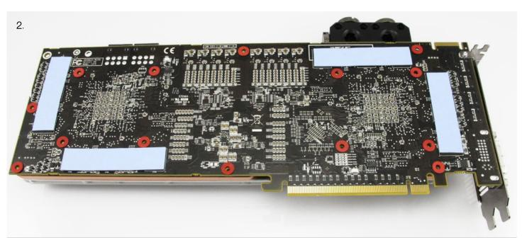
2. Flip the card over, making sure the front thermal pads stay in place. Now remove the tape from both sides of the rear thermal pads and place them on the positions shown above. Place the red washers over the screw holes shown above.
