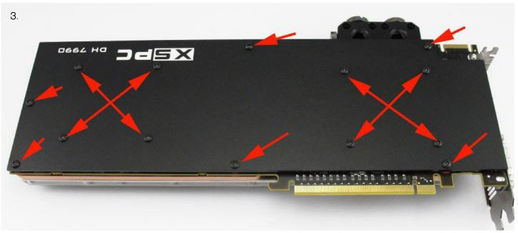
**3**. Place the backplate on the back of the card and attach it using the black M3 screws. You should start with the eight screws behind the GPU's. Do not over tighten the screws as this may bend the card and cause permanent damage.
